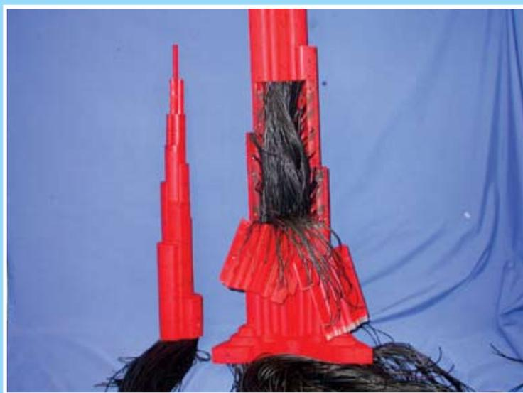
Figure 4: Detail of Pressure Taps in Cladding Pressure Test Model
