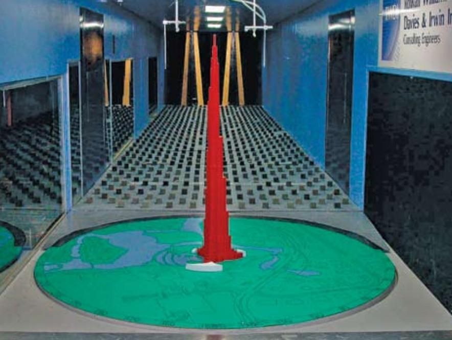
Figure 3: Cladding Pressure Test Model at 1:500 Scale, Shown in Wind Tunnel
