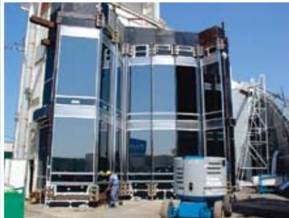
Figure 6a: Tower Test Mock-up Assembly.
