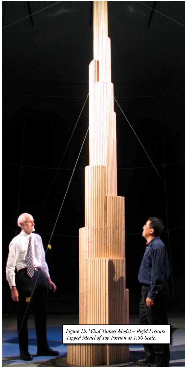
Figure 1b: Wind Tunnel Model – Rigid Pressure Tapped Model of Top Portion at 1:50 Scale.
