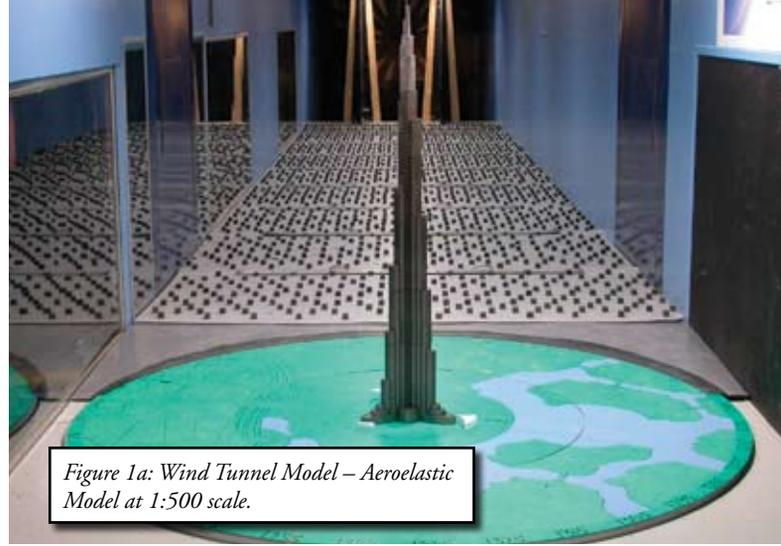
Figure 1a: Wind Tunnel Model – Aeroelastic Model at 1:500 scale.
